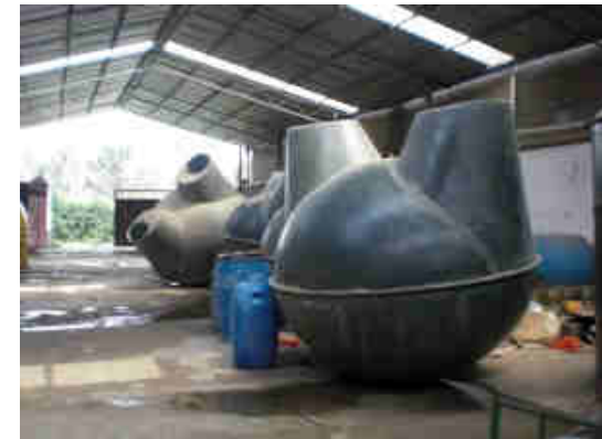
Fibreglass reinforced plastic digesters
